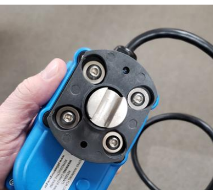
4_Mounting plate and stem coupling in place
