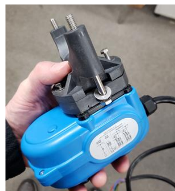
6_Attach top bracket to mounting plate using screws and washers
