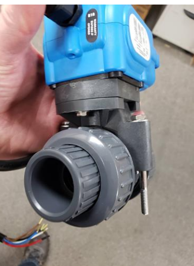
7_Top section mounted to actuator. Nest the valve stem into stem coupling through the top bracket
