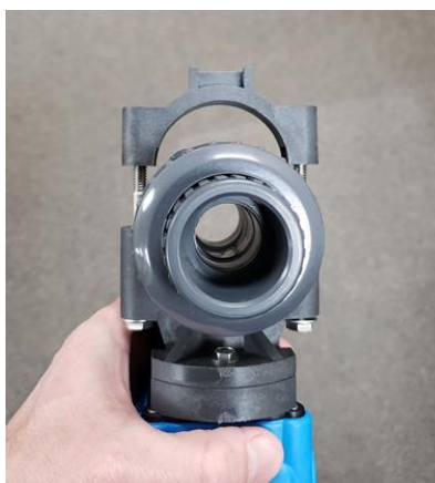
8_Attach bottom bracket. You may have to squeeze it to align with screws. Use washers and Nylock Nuts.
