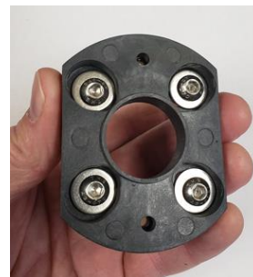
3_Washers and button screws in mounting plate
