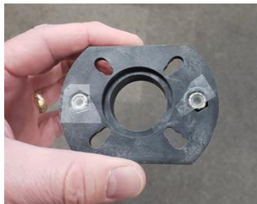
2_Put Nylock nuts in place in mounting plate and put tape over them
