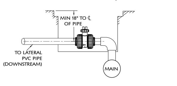
\*2-1/2" is 3" valve with reducing end connections
